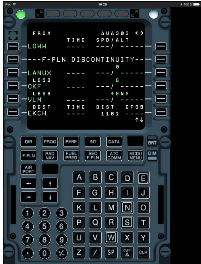
Screenshot of the MCDU taken on an iPad using the Chrome browser
